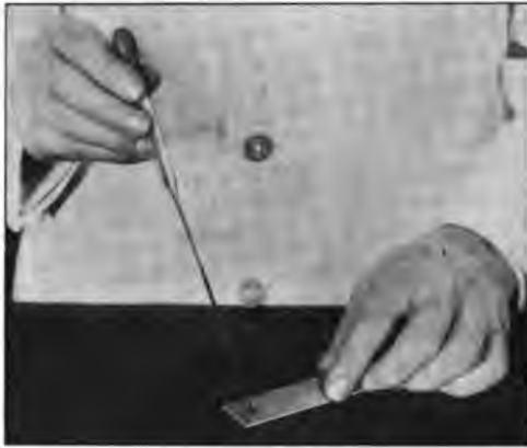
Fig. 98.—Mixing liquids by repeatedly expelling on to slide and redrawing into pipette (Miller).
